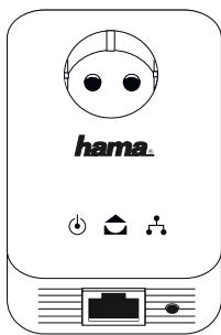
Insert the second Powerline adapter (B) into an empty socket.
